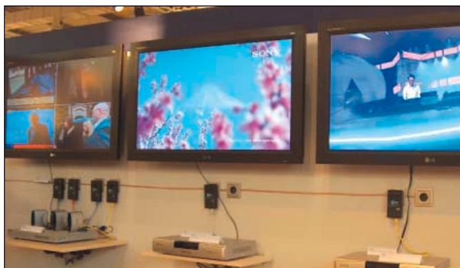
This is DS2's demonstration of its 200Mbits/sec data-over-mains technology. The two screens on the right are showing 25Mbits/sec high-definition video streams and the other windows four standard TV streams - all delivered over a single mains link via the plug-in DS2 modems visible beneath the displays. Corinex ( www.corinex.com ) says it will be selling a €90 (£62 approx) DS2-based modem in the UK within a couple of months
